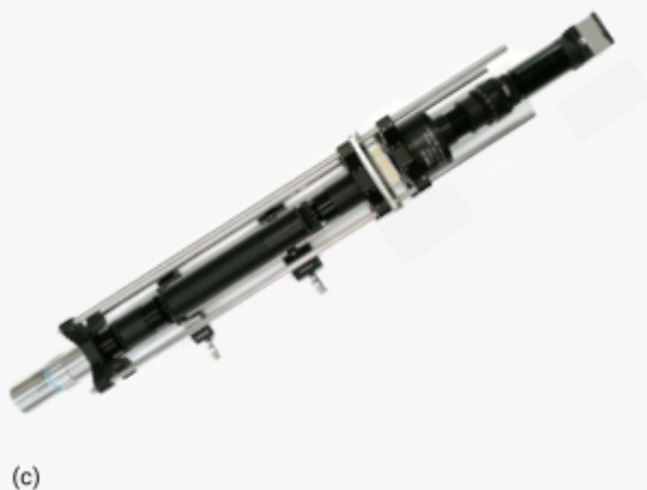
Figure 5: Examples of DPP-based AO systems in commercial and custom-built microscopes. (a) DPP integrated between the objective and turret of a commercial microscope. (b) DPP integrated at the conjugate pupil plane of a commercial microscope using a relay optic attached to the camera port. (c) 'World's smallest AO microscope' for fluorescence wide-field imaging [5]. (d) DPP integrated to the illumination path of a custom-built two photon microscope (in collaboration with the group of Prof. Alexander Jesacher, Medical University of Innsbruck)[10].
