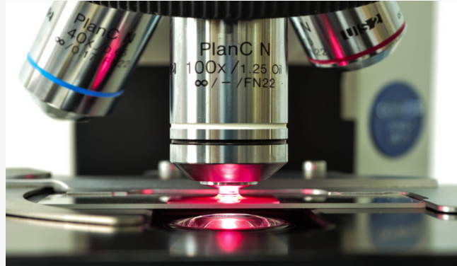
Figure 1: Oil / Water immersion microscopy setup.
