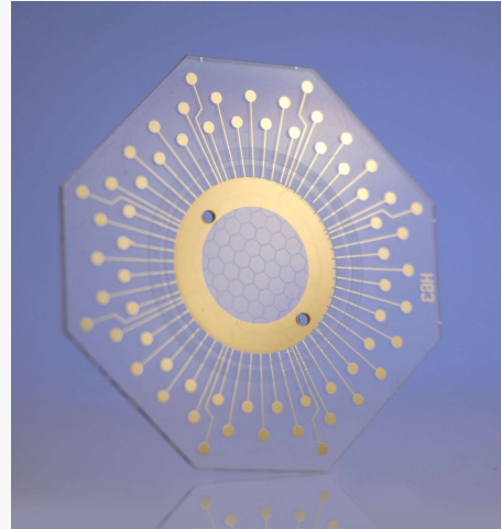
Figure 4: Refractive 63-actuator Deformable Phase Plate, able to correct for 7 th radial Zernike order.
