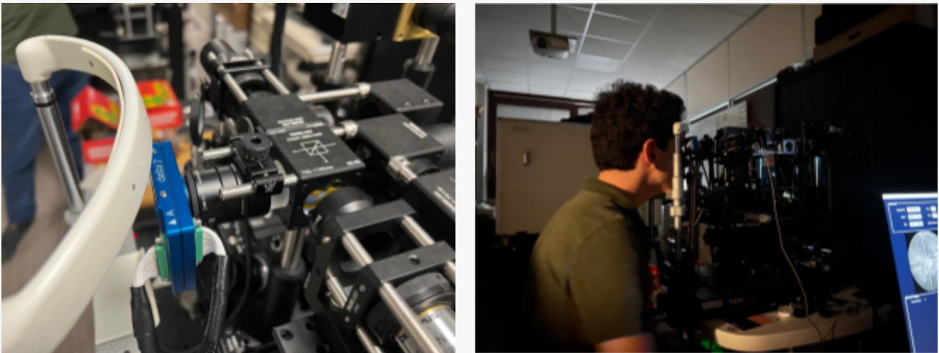
Figure 3: Retrofitting Phaseform's refractive AO system to an existing full-field OCT ophthalmoscope at the Institut Langevin. The only hardware change that was necessary for the AO upgrade was to introduce a DPP after the last lens in the system that is placed in front of the patient's eye (left). By feeding the instrument's image data into Phaseform's AO sensorless wavefront estimation algorithm, the integration was complete. The imaging workflow after AO integration remained mostly intact, the only exception being the aberration estimation step, which took about 3 seconds. The rest of the retinal image acquisition procedure proceeded as usual.
